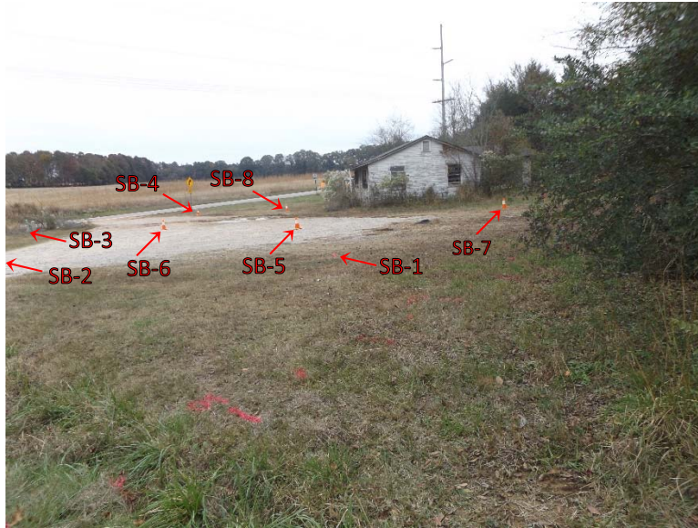
Photograph 2. Eastern portion of investigation area showing GeoEnvironmental soil boring locations W-5710Y.4-SB-1 through W-5710Y.4-SB-8.
